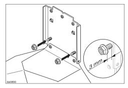
■ First loosely screw the two locking nuts onto the threaded bolts on retaining plate A.
